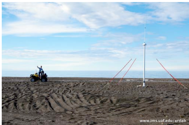
Figure 1: Receive antenna for the SeaSonde system on the right. A person atop an all terrain vehicle is on the left for scale
